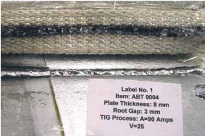
Close-up of the weld bead achieved with Light Duty Weld Backing Tape. 8 mm Plate, 3 mm Root Gap, Manual TIG Process at: 90 Amps, 25 V
