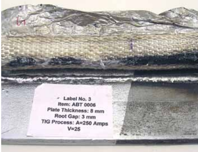
Close-up of the weld bead achieved with Heavy Duty Weld Backing Tape. 8 mm Plate, 3 mm Root Gap, TIG Process at: 250 Amps, 25 V
