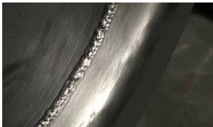
Step 3: Remove the tape to see a flat, well formed bead
